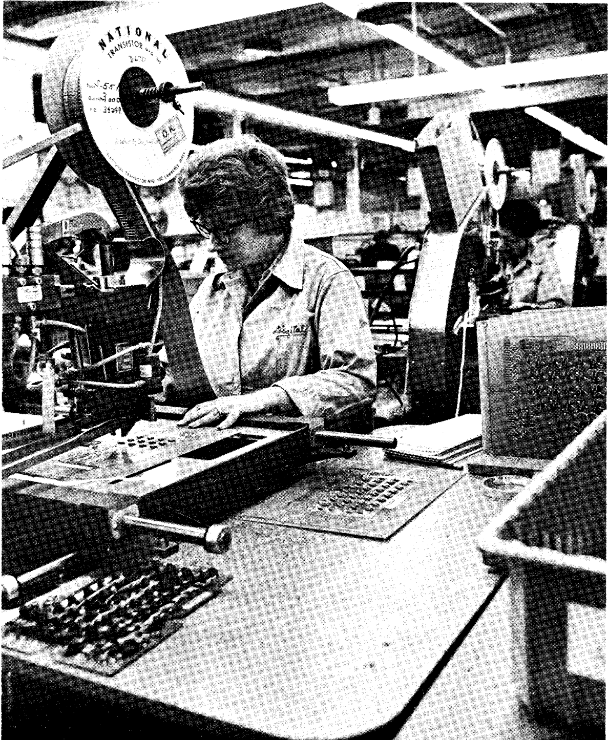
Discrete components are positioned and crimped in place at rates up to 30 per minute on pantograph controlled inserting machine.
